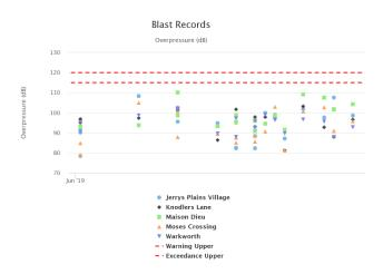
Figure 81: Overpressure Blast Monitoring Results – June 2019
